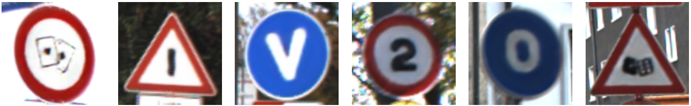
Fig. 5. The depicted traffic signs show the ability of our method to generate realistic looking images from arbitrary (including fictitious) traffic sign icons. Resulting images show adaptation in illumination, pose and motion blur as would be expected from natural traffic sign images.
