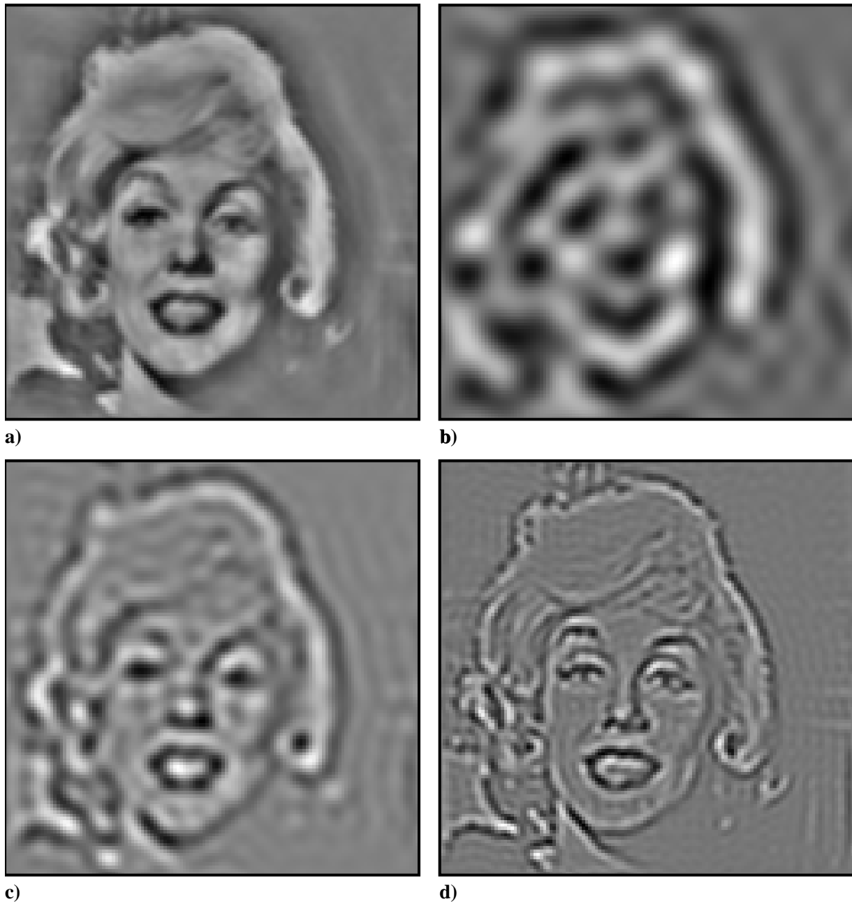
Figure 3.5: Reconstruction from single frequency levels. Picture a) shows the reconstruction from the full representation, b) from \mathcal{K}_0 , c) from \mathcal{K}_1 and d) from \mathcal{K}_2 only.
