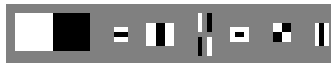
Figure 4: Optimized feature set. The features have sizes of 16 \times 8 , 3 \times 3 , 6 \times 5 , 3 \times 9 , 4 \times 3 , 4 \times 4 , and 3 \times 5 .
